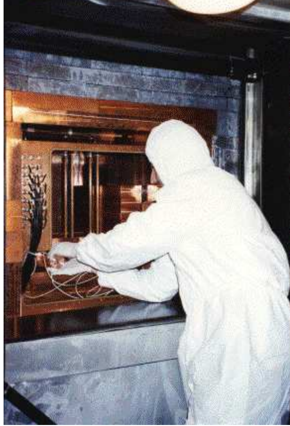
DAMA experiment: Installing the detectors inside the copper box and shield
