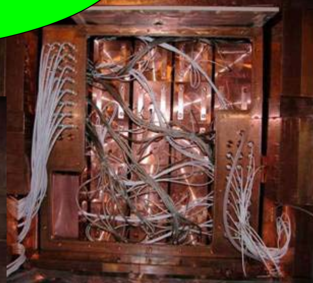
view at end of detectors' installation in the Cu box
