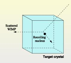
Direct detection through the elastic scattering of a WIMP with nuclei inside a detector.
